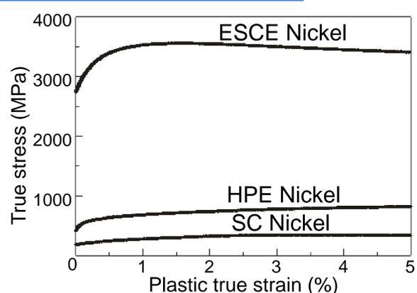
Yield strength of ESCE Nickel is 10 times higher than SC & 5 times higher than HPE
